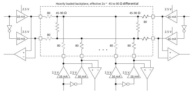
Figure 3.2. BLVDS Multi-point-Output Example
