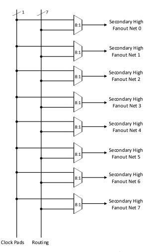
Figure 2.5. Secondary High Fanout Nets for MachXO3D Devices
