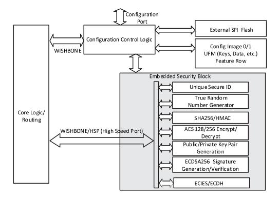
Figure 2.16. ESB Core Block Diagram
