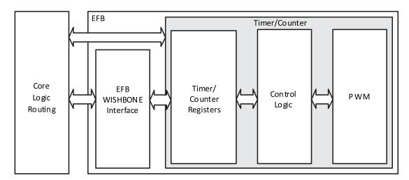
Figure 2.19. Timer/Counter Block Diagram
