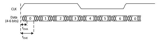
Figure 3.6. Receiver GDDR71\_RX. Waveforms
