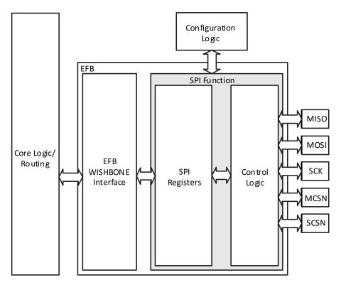
Figure 2.18. SPI Core Block Diagram
