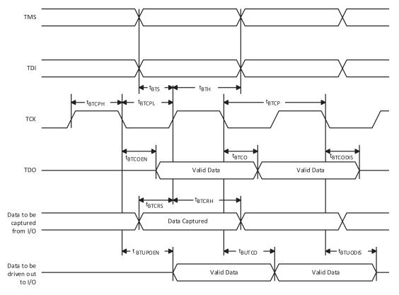
Figure 3.8. JTAG Port Timing Waveforms
