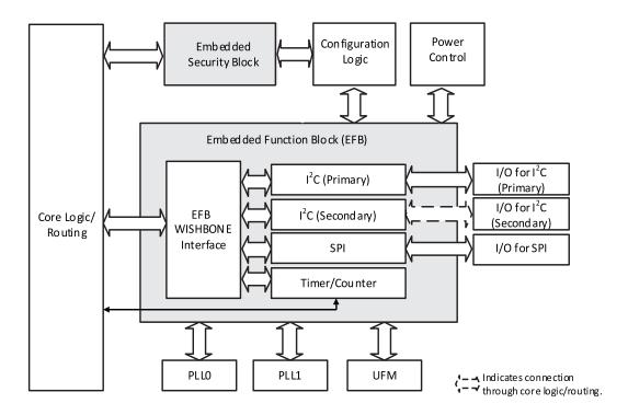
Figure 2.15. Embedded Function Block Interface
