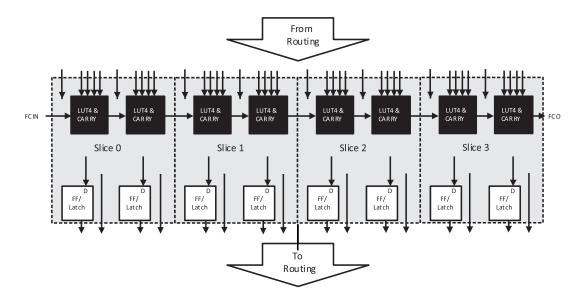
Figure 2.2. PFU Block Diagram
