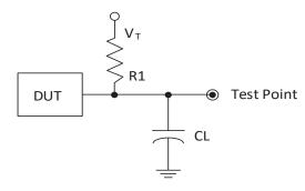
Figure 3.9. Output Test Load, LVTTL and LVCMOS Standards
