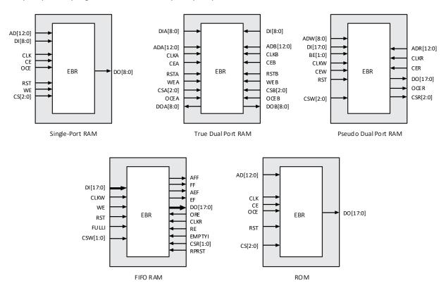
Figure 2.7. sysMEM Memory Primitives
