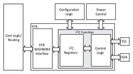
Figure 2.17. I<sup>2</sup>C Core Block Diagram
