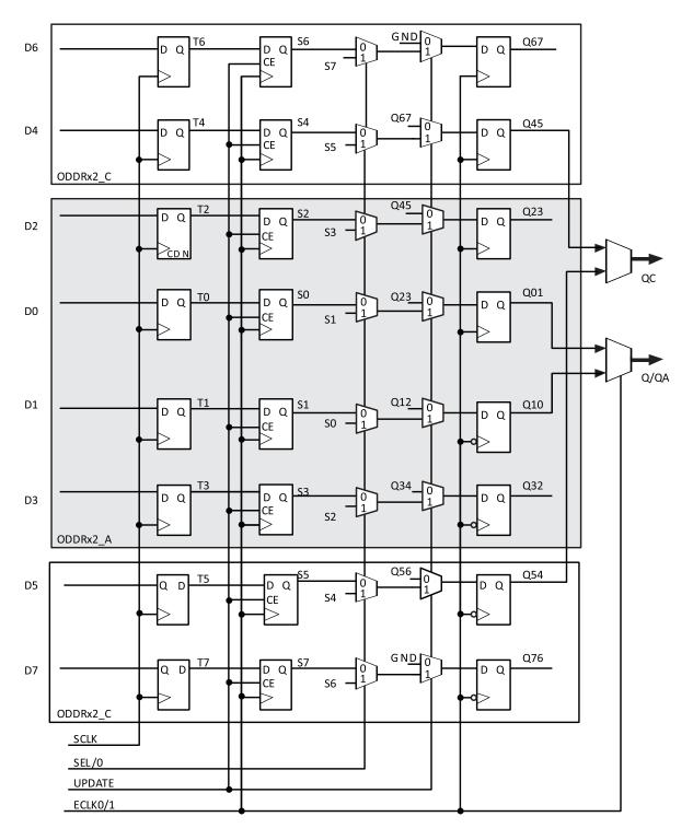
Figure 2.13. Output Gearbox
