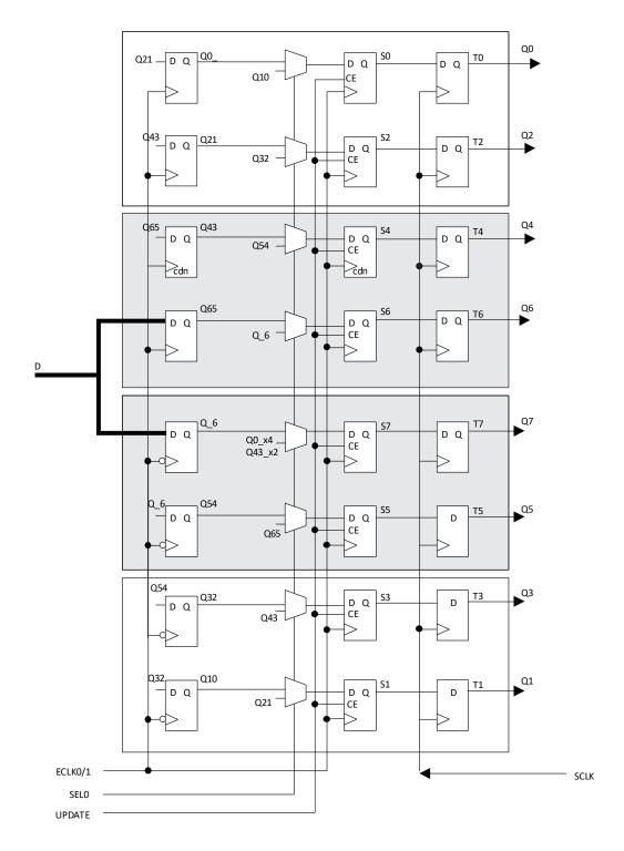
Figure 2.12. Input Gearbox
