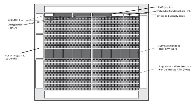
Figure 2.1. Top View of the MachXO3D Device
