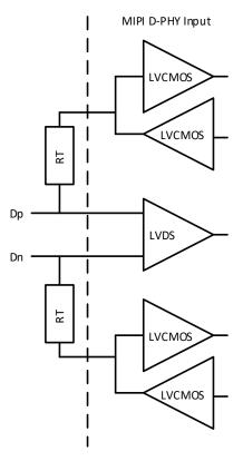
Figure 3.4. MIPI D-PHY Input Using External Resistors
